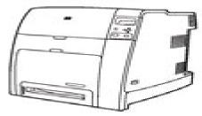
The HP Color LaserJet 4700 printer is a four-color laser printer that prints up to 31 pages per minute (ppm) for letter-sized paper and up to 30 ppm for A4-size paper.
