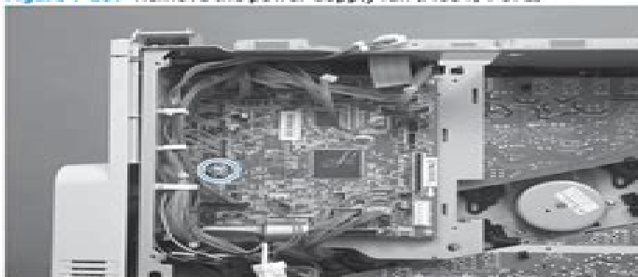
Figure 1-297 Remove the power-supply fan (M651; 1 of 2)
