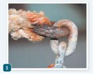
5. Watch for abrasion and corrosion at the splice. This link needs to be tossed out.
