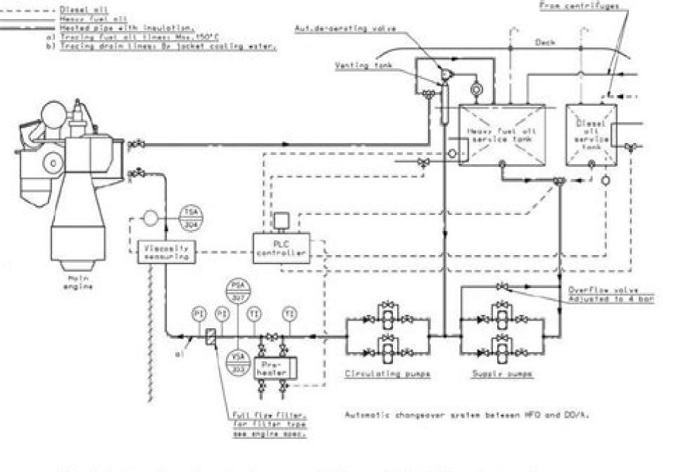
Fig. 6: Automatic system for changeover between fuels of different viscosity
