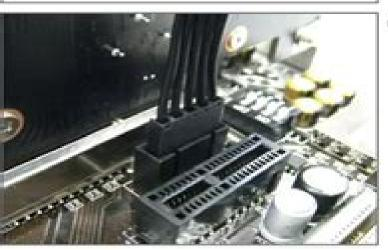
(Note 1) The Thunderbolt™ header cable (5-pin) provided has two connectors. Choose the correct connector according to the Thunderbolt™ add-in card header on your motherboard.
