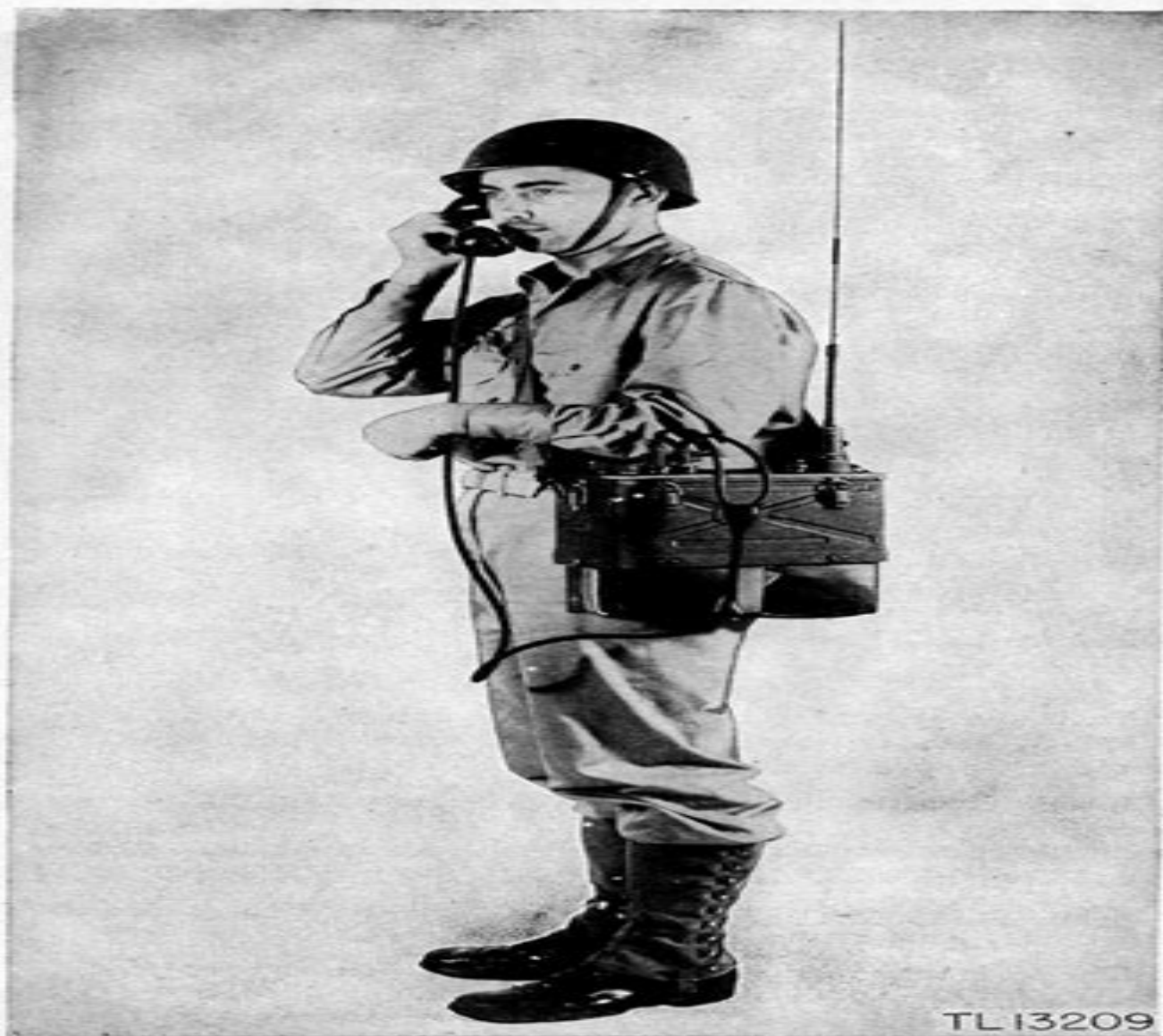
Figure 19. Radio Set SCR-300-A, lightweight installation.
