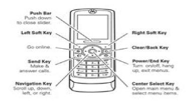
Tip: Press the center key + to open the main menu and select menu options. Press the clear/back key
