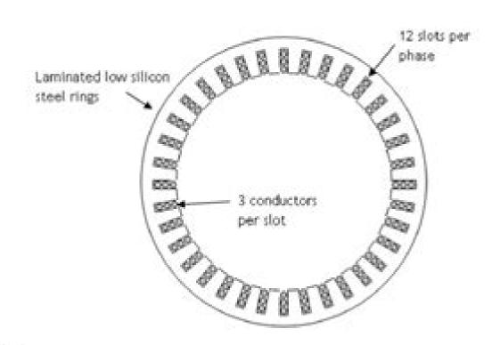
Example of 36 slot stator
