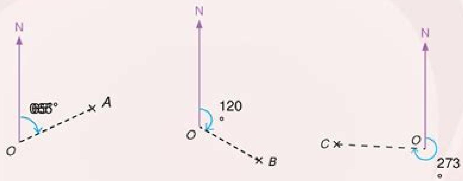
The true bearings of *A*, *B* and *C* measured from *O* are 065°, 120° and 273° respectively.
