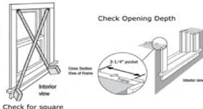
Measure and record the width between the side jambs at the bottom, middle and top of the window. Raise the sash to take the measurements. If necessary, remove jamb liners and weatherstripping to get an accurate measurement. Record the smallest width. It is important to measure in all three places to be sure the opening is square.
