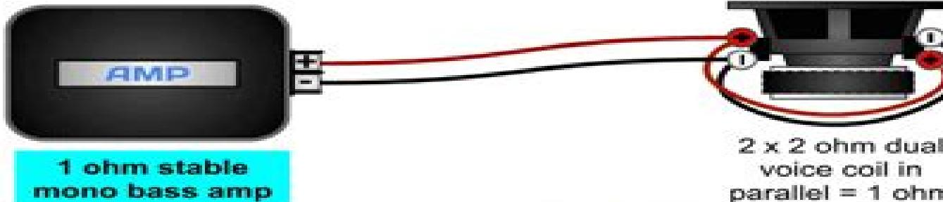
2 x 2 ohm dual voice coil in parallel = 1 ohm
