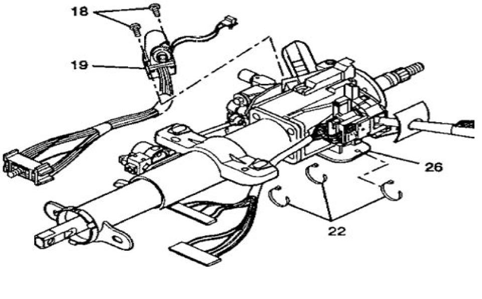
18 SCREW, TAPPING 19 SWITCH ASM, IGN & KEY ALARM 22 STRAP, WIRE HARNESS 26 HOUSING ASM, STRG COLUMN
