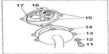
Fit spring plate (17) and lever guide (16). Secure with screws (15). Position new gasket (14) and cover (13) over the valve chest and secure with screws (11) and washers (12).
