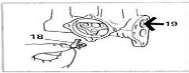
Insert 'T' lever valve (18) and press in plug (19) to allow round end of lever to fit easily into the hole in control piston.
