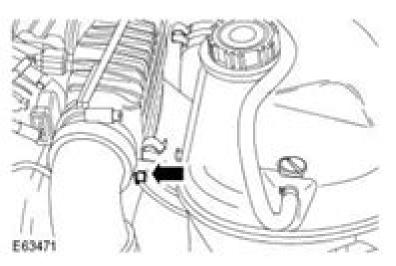
3. Remove the intake air shutoff throttle elbow retaining bolt.
