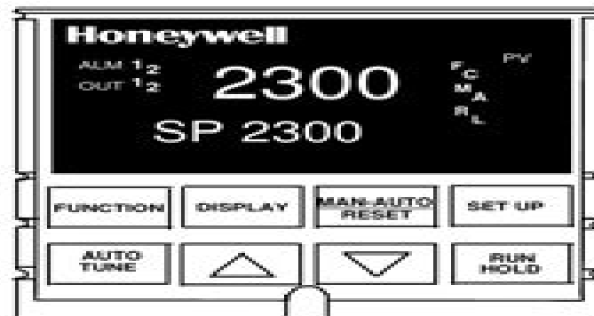
Figure 1—UDC 2300 Controller has a sealed faceplate suitable for hosedown applications
