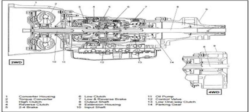
Figure 1. Construction of Automatic Transmission
