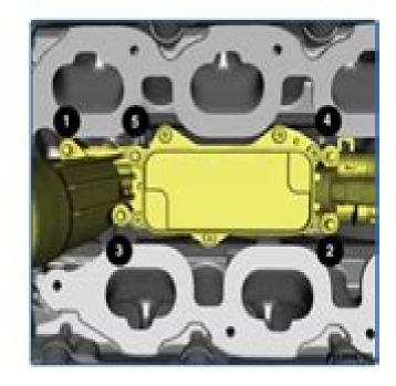
5. Install the heater hase (1) to the oil filter housing.
