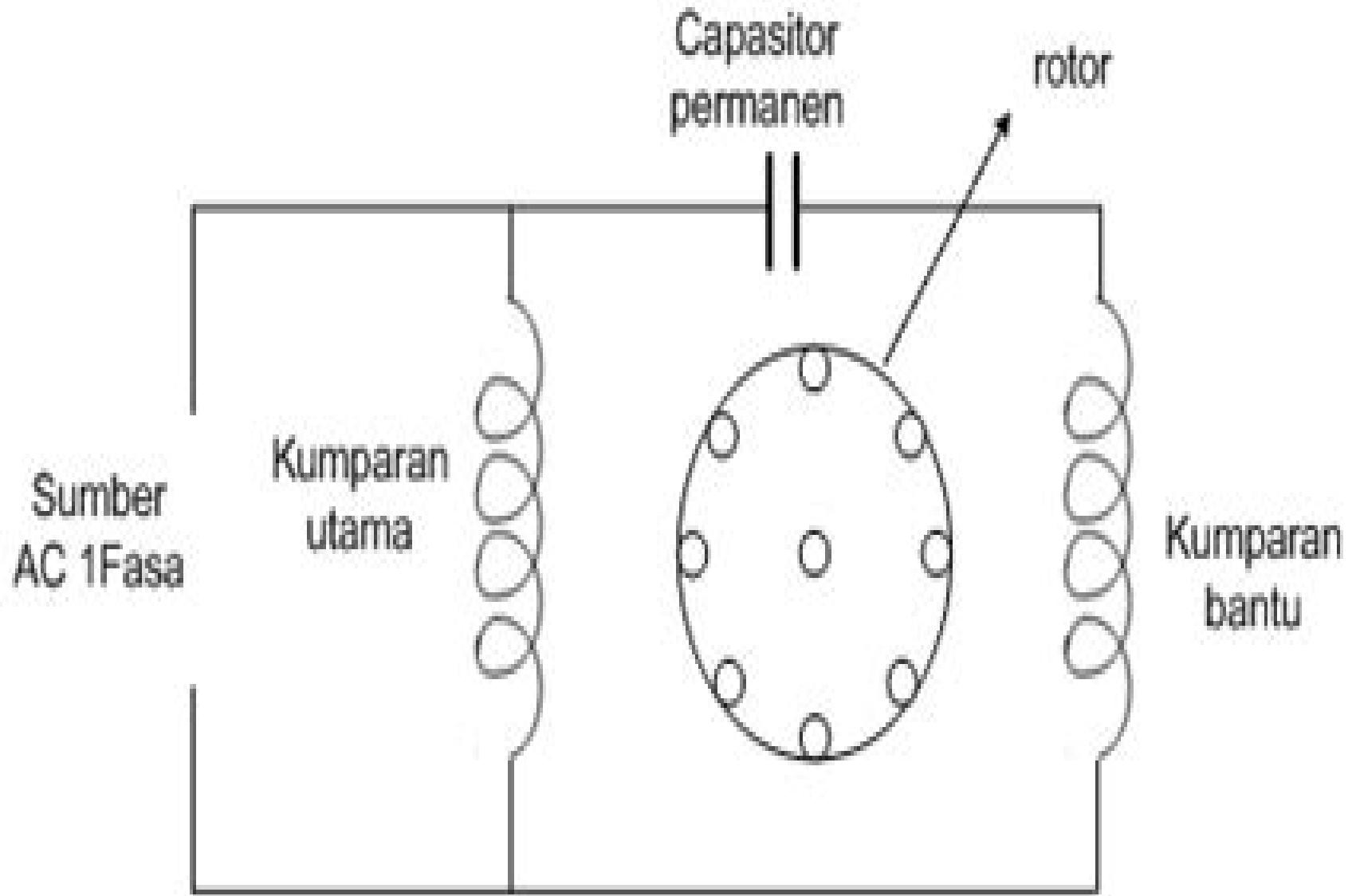
Gambar 04. Motor running kapasitor
