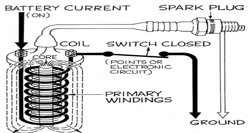
STRONG MAGNETIC FIELD BUILDS AROUND COIL AND PRIMARY WINDINGS
