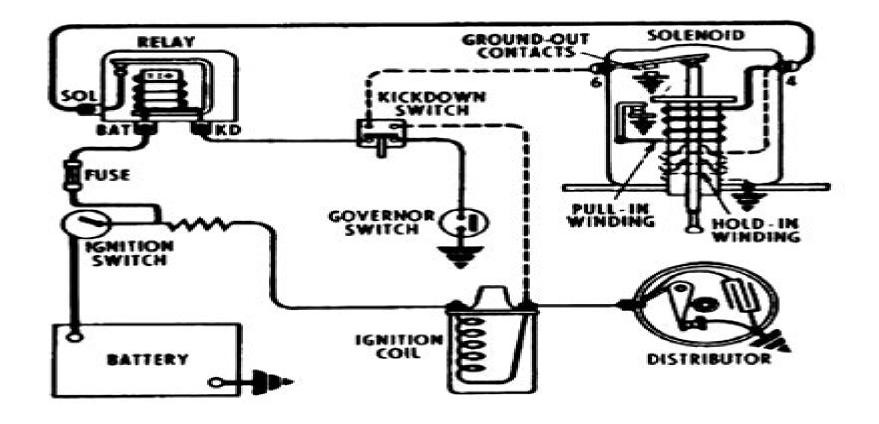
Overdrive Electrical Circuit Wiring Diagram
