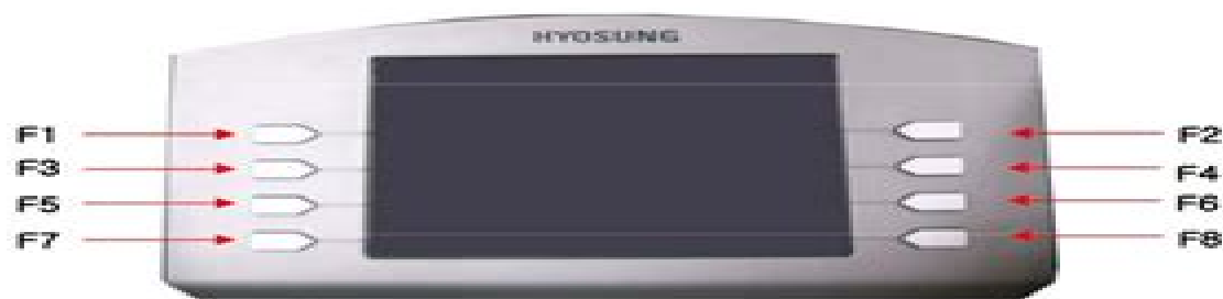
- Function Key Location on ATM -
