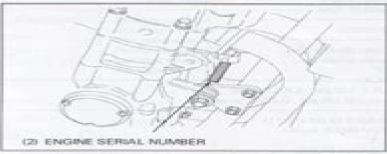
The engine serial number is stamped on the front of the lower crankcase.
