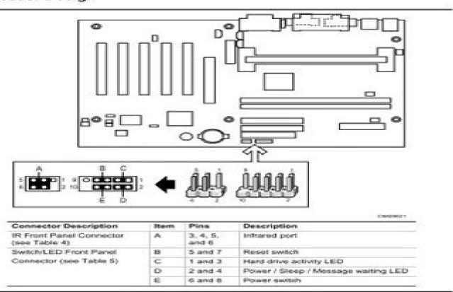
Figure 1. Front Panel Switch/LED and IR Headers
