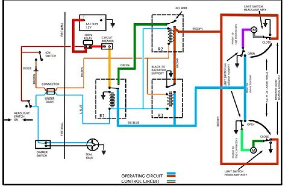
67 CAMARO HEADLAMP DOOR WIRING - SYSTEM IN "HEADLIGHTS ON DOORS OPEN" POSITION
