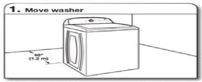
Move washer to within 4 ft (1.2 m) of its final location; it must be in a fully upright position.
