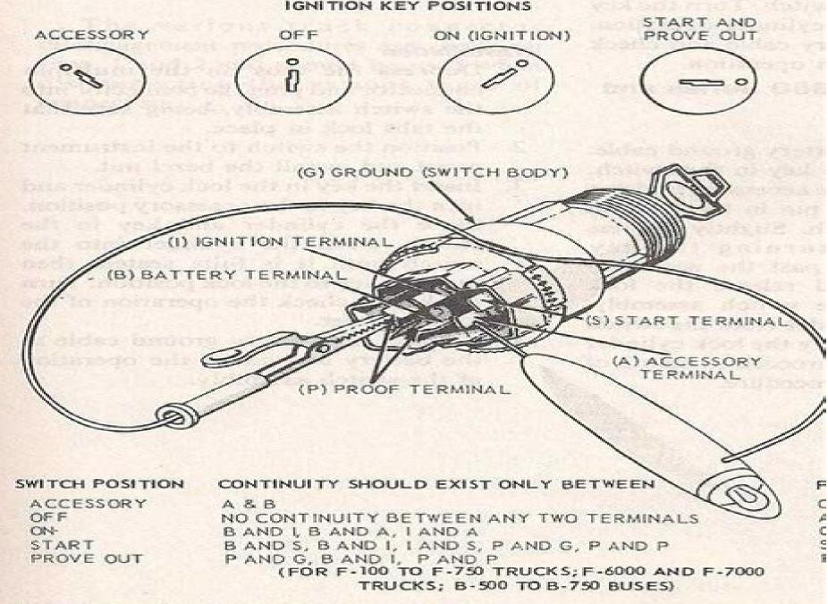
FIG. 1 Ignition Switch Continuity Test
