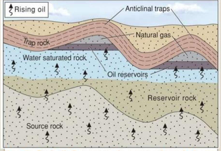
How to find oil: Source rock, reservoir rock, traps
