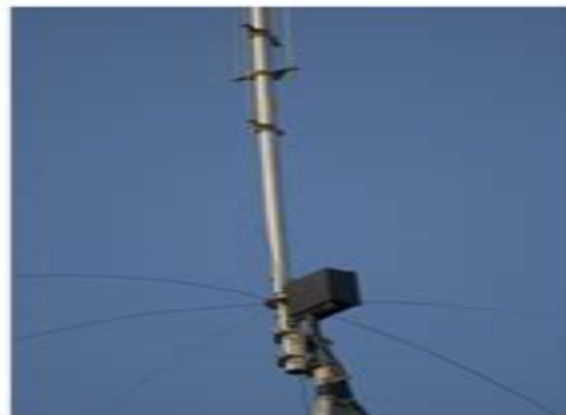
Matching network and base of stubs
