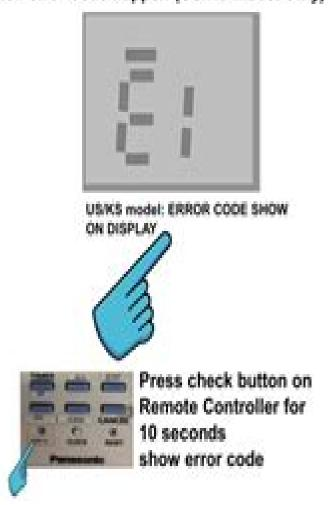
After repairing, blinking would stop and error code disappear.
