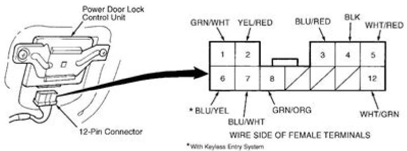
Disconnect the 12-Pin connector from the power door lock control unit.
