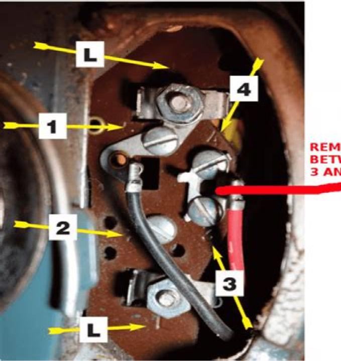
REMOVE THE 2 PLATES BETWEEN TERMINALS 3 AND 4
