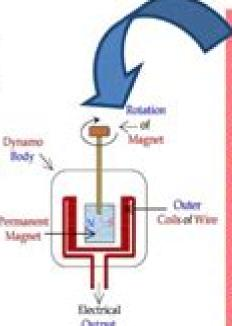
Bicycle dynamos work by electromagnetic induction. As the rider pedals, a permanent magnet turns inside a coil of wire. The rotating magnet changes the magnetic flux linking the coil. An emf is therefore induced.
