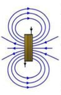
With a coil, we can think of the number of field lines linking the coil. If there is a change in the number of field lines which pass through the coil, there will be an induced emf across the ends of the coil.
