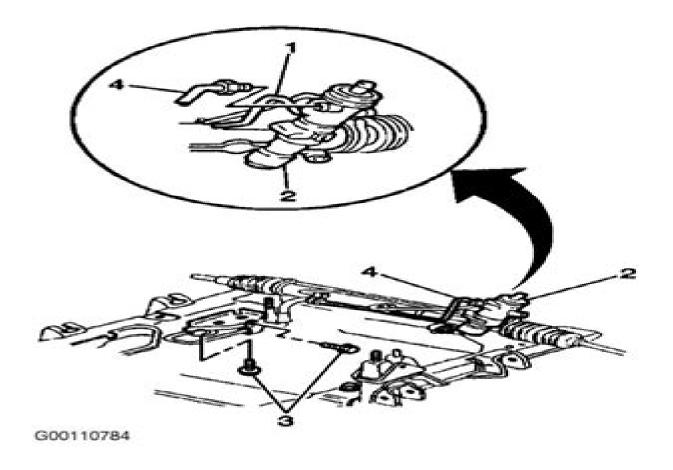
Fig. 2: Removing Power Steering Return Line From Power Steering Gear Courtesy of GENERAL MOTORS CORP.
