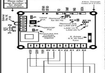
WOLTS: House thes e pot clockwise to increase AC terminal voltage and anticlockwise to decrease AC terminal voltage. If it is required to adjust generator voltage from remote location then a 1 K/1 W potentiometer can be connected in series with sensing phase R of AVR. Using 1 K potentiometer voltage can be varied in the
