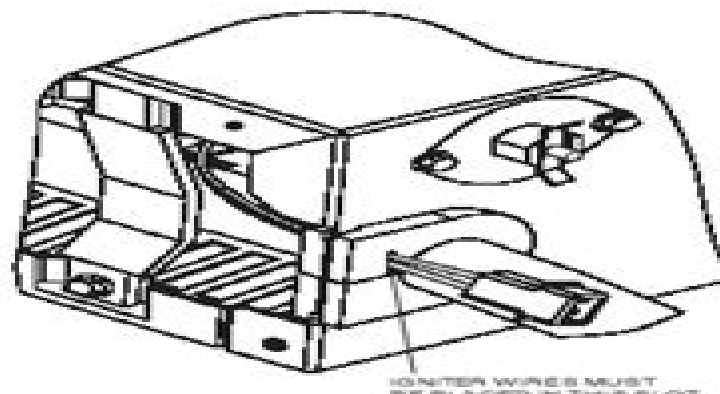
Fig. 7 - Igniter Wire Placement
