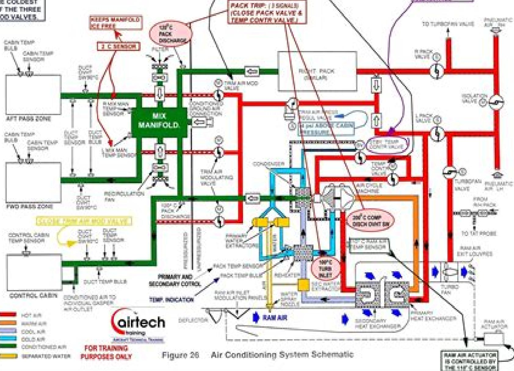
**Figure 26** Air Conditioning System Schematic
