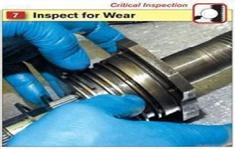
Replace all iron sealing rings. Inspect the governor distributor contact surfaces inside for wear prior to tailshaft installation.
