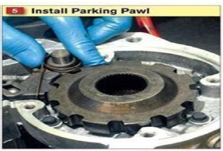
The installed parking pawl, return spring, and gear.
