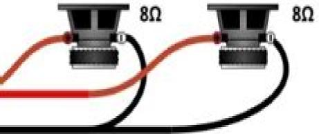
's connected in parallel divide their impedan Ohms):  $8\Omega / 2 = 4\Omega$
