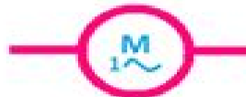
Single Phase Motor Symbol
