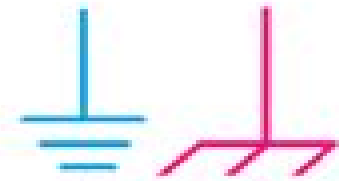
Grounding or Earthing Symbol
