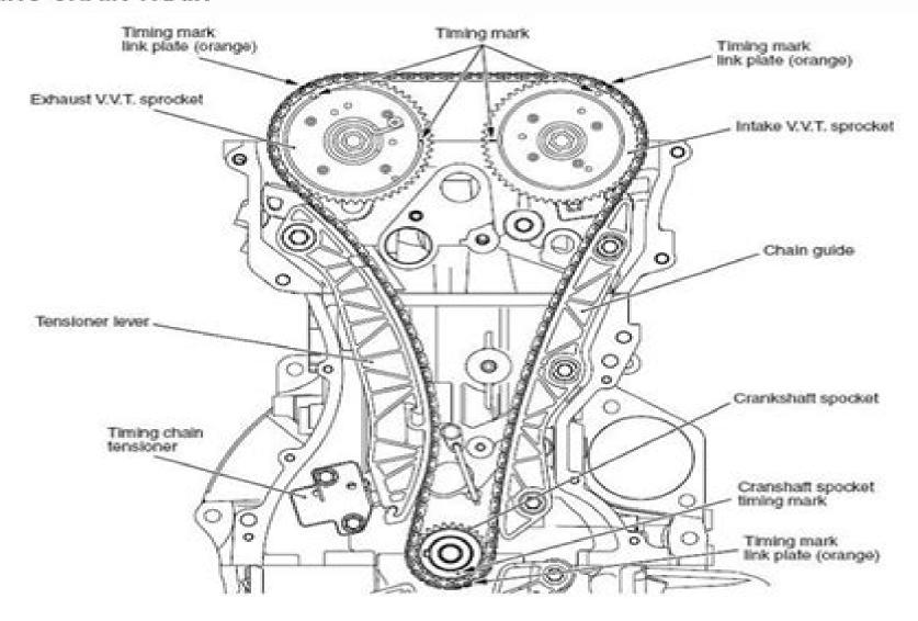
The two camshafts are driven by the timing chain via the camshaft sprockets.
