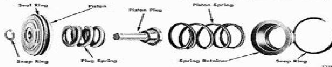
FIGURE 98 — Low-Reverse Servo Assembly Sequence
