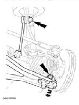
CAUTION: To avoid to damage joints and boots, do not bent the inner halfshaft joint by more than 18 degrees, the outer one by not more than 45 degrees.
