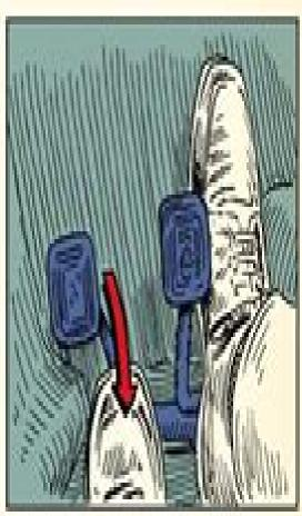
Once in gear, keep foot off clutch.
