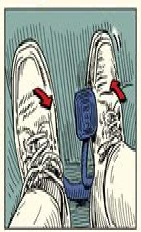
Remove left foot from clutch while pressing on the gas pedal with right foot.
