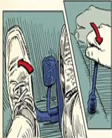
Take your right foot off the gas pedal, press in the clutch completely with your left foot, and shift into a lower or higher gear. This should be done in one synchronized motion.
