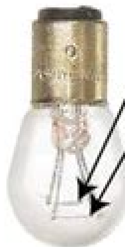
Thicker filament for brake light
