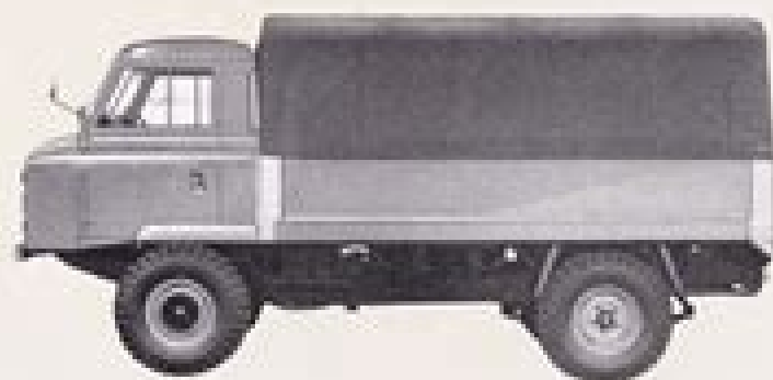
With truck cab, fixed-side body and full-length hood.
