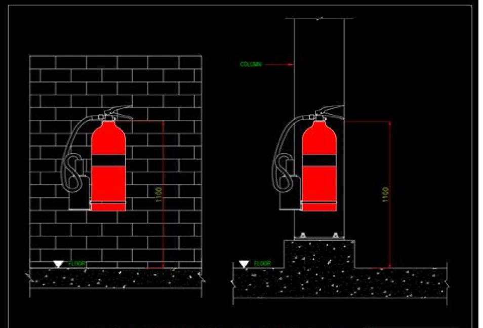
TYPICAL INSTALLATION DETAIL FOR CO2 FIRE EXTINGUISHER WGShare.com
