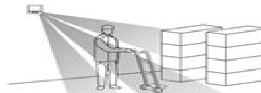
Figure 4. Blocking coverage pattern
