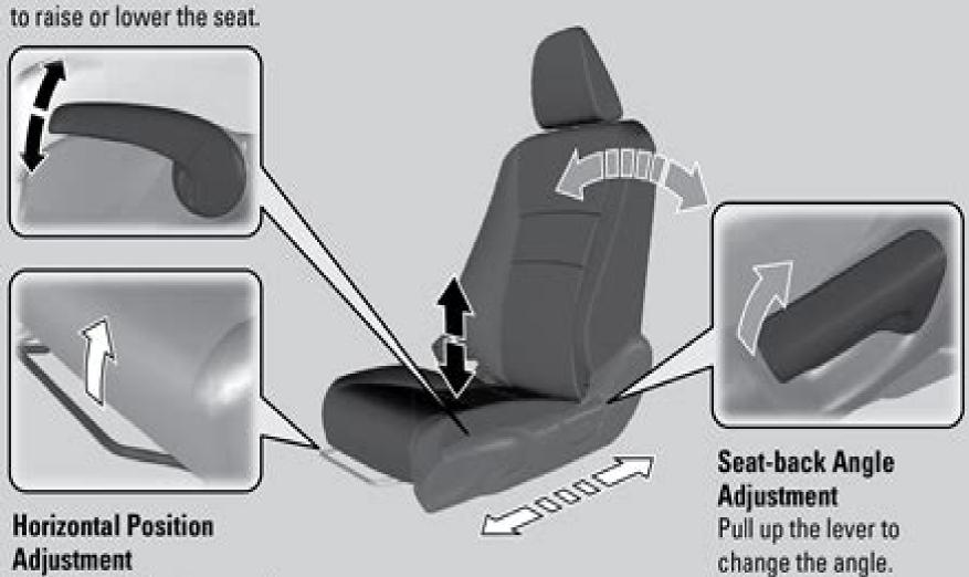
Pull up on the bar to move the seat, then release the bar.
