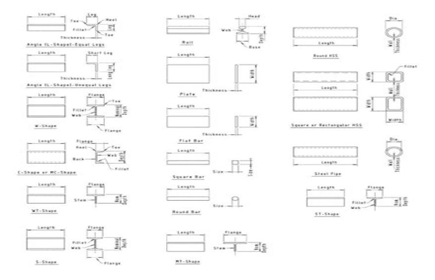
Figure 1-1. Typical cross-sections of raw steel material.
