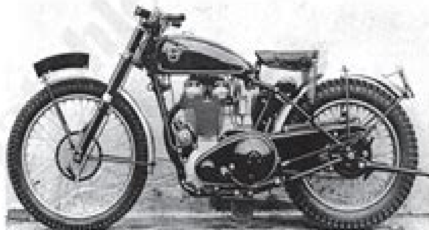
A maker's definitive photograph by courtesy of Matchless (specifies the 1955 500cc Matchless G50) shown here in main gear with 14" wheels, main, pre-Matchless carburettor, rigid frame, Barmen box and the L&L style of forward-mounted magneto introduced (late September 1954. The Lucas magneto box is of course the "Walter" type. It has the side-appe from brake brought in September 1952, the fullbrake from but not arriving until 12 months later.
